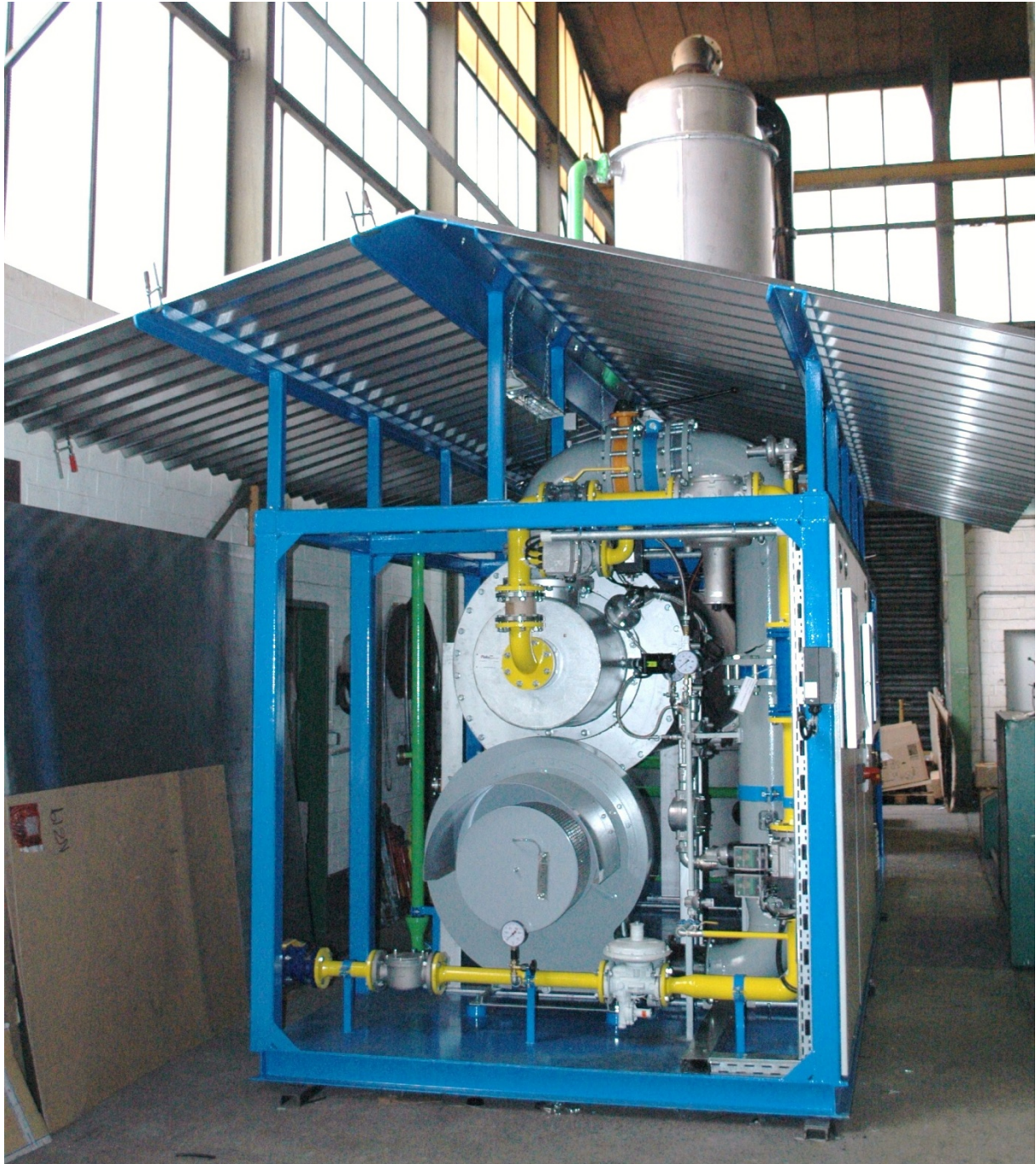
Big-size exothermic generator type EXOLEN with a production capacity of 3.500 Nm 3 /h
