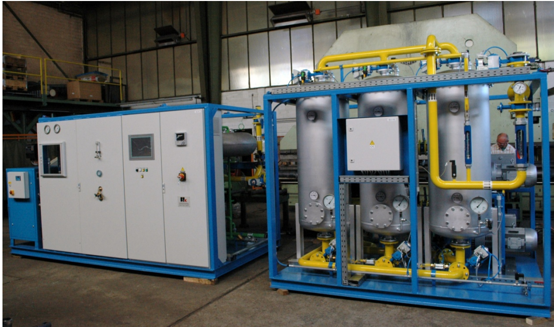
Complete Monogas unit, consisting of Exo-gas generator type EXOLEN and dryer type PURILEN
